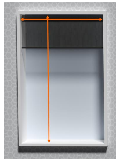
figure 1: measuring an inside fit roller blind
